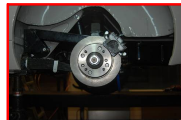
Fig 4 New caliper & disc fitted correctly on the axle
