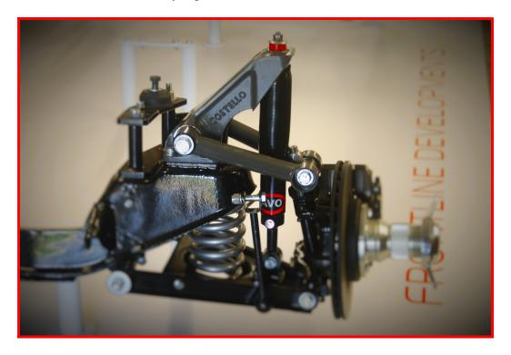
The conversion kit consists of a pair of precision-machined LM25 aluminium top bracket and tubular wishbone arms, bespoke Avo adjustable telescopic dampers, lower damper mounting brackets and a fitting kit.
