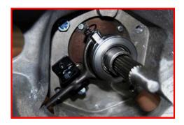
(*Note:* check the pivot bolt & the bearing in the clutch fork for wear as this may impair the clutch travel and operation.) Tighten to remove side play but do not impair lever action. (**See notes on clutch release bearing**).
