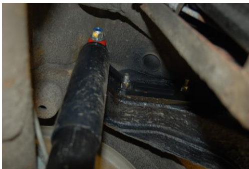
Right hand top damper mounted
